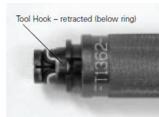
Figure 3 – O-ring & Back-up ring Loaded Into Tool
