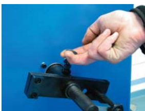
Easy tool exchange using a locking pin
