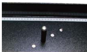
Steplessly adjustable length stop
