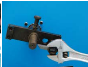
External Skiving Preset each of the eleven external skiving tools once for each hose diameter you need
