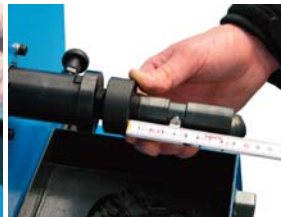
Internal Skiving Easy setting for a fixed stop for internal skiving
